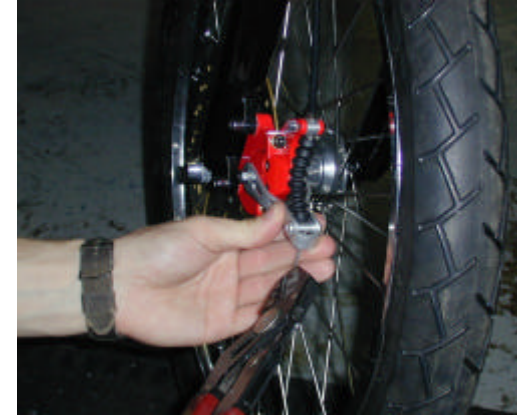
Brake Tensioning Step 2: Brake cable pulling
