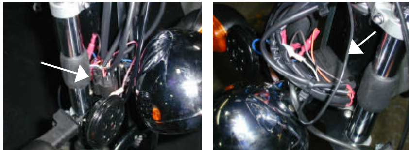
Step 10: Connector in vertical position (left) and horizontal position (right)
