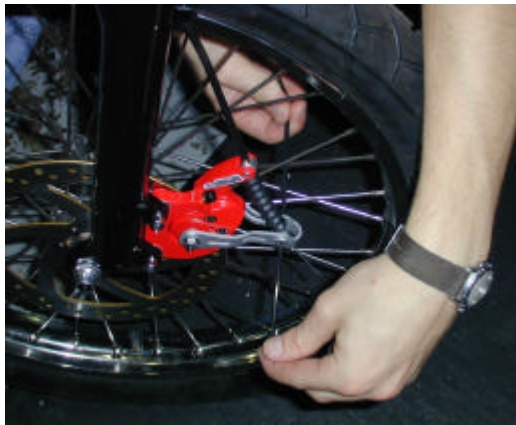
Brake Tensioning Step 1: Brake cable clamping mechanism
