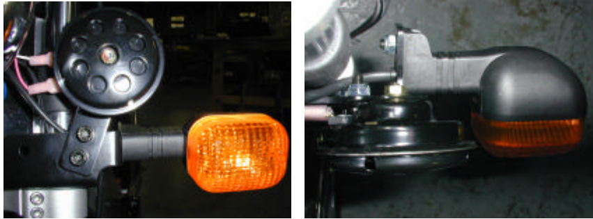
Step 4/5: Installation position for horn and directional on front end of Voloci
