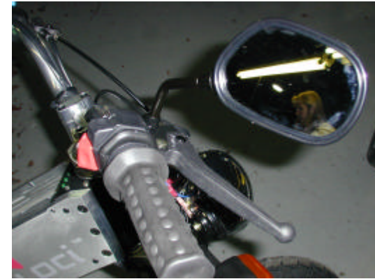
Step 19: Mirror mounted on right brake housing
